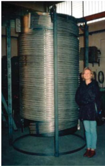
Prototypic bundle, developed originally for a 20 MW thermal reactor and of the same diameter as the IRIS steam generator, was fabricated and tested
