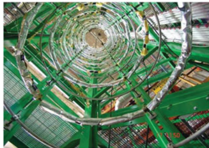
IETI (SIET Italy) Facility Thermal-Fluid-Dynamics experiments on a full-scale helical-coil tube of the IRIS reactor steam generator
